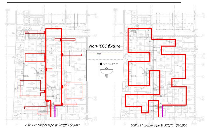
Serpentining large supply pipes overhead is a common practice as a method of positioning the water supply as close to the fixtures as possible to avoid lengthy runouts/dead legs. This method can be costly adding hundreds of feet of pipe length, surface area and volume to the installation.
